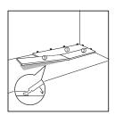
Then raise the newly installed plank to an angle of 20°-30°. This will also raise the previously installed planks in the same row, because their short sides are already connected.
